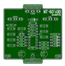
Mainboard Dimensions – 2.10" x 2.12" – Perfectly sized for a 1590B or 125B enclosure
