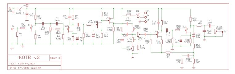
The Master control is a post-EQ control that helps attain even higher levels of saturation prior to hitting the stage at Q5 and the Level is an overall volume control of the entire circuit. There is a subtle difference between the ranges of distortion since a cranked amp is what this is designed to produce and delivers in spades! This circuit does not produce clean or low-gain tones.
