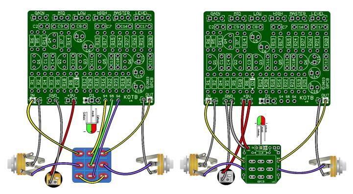
Note: Status LED can be mounted to the main board or 3PDT wiring board if used. Choose your favorite location.
