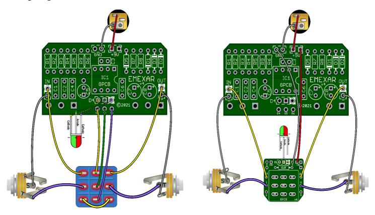
If you are using our 3PDT board, you should omit wires and parts from S4, S5 & S6, D4 and R9 (CLR). The CLR and LED will be populated on the 3PDT board instead.
