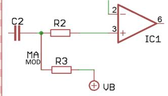
\*The MicroAmp™ has a single Level control. Use a fixed 10k resistor soldered between "Volume" pads 1 and 2, and a jumper between pads 2 and 3.
