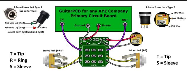
Multiple +9v and Ground Pads are convenient hookup points for additional circuits within the same enclosure. This also allows for diverse wiring schemes to suit indiviual needs.
