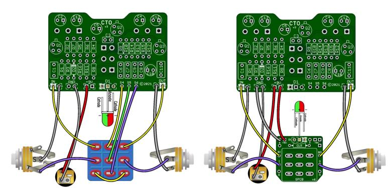
Build Notes: If you are using our 3PDT board, you should omit wires and parts from S4, S5 & S6, D1 and R16 (CLR). The CLR and LED will be populated on the 3PDT board instead.
