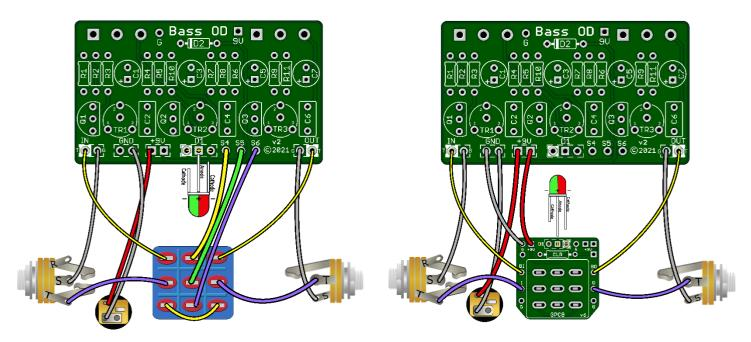
Build Notes: If you are using our 3PDT board, you should omit wires and parts from S4, S5 & S6, D1 and R10 (CLR). The CLR and LED will be populated on the 3PDT board instead.
