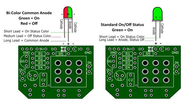
Insert the LED leads into the corresponding pads as shown above. If you wish to change the color of the On Status then simply flip the LED to change to the cathode of the color you wish to use. R5 is the Current Limiting Resistor. Use a value from 1k8 to 4k7.
