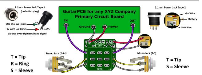
Multiple +9v and Ground Pads are convenient hookup points for additional circuits within the same enclosure. This also allows for diverse wiring schemes to suit individual needs.
