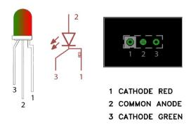
The diagram above shows the pin-out, schematic symbol and pad connection for a common anode LED. The pin-out for the bi-color LED is as follows:
