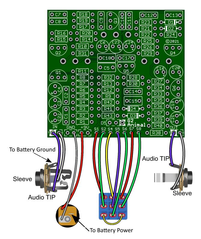
The standard circuit employs a buffer stage (Q1 stage) that is permanently connected even when the circuit is in bypass mode i.e., the circuit is not a true bypass system. Because of this you do not use a 3PDT Wiring Board with this circuit. Also, we recommend using the on-board LED pads (D5) as well for your status LED.
