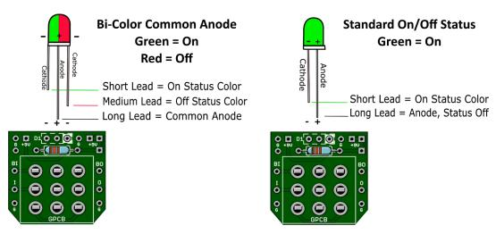
Note: If wiring the LED to our 3PDT board no need to connect S4, S5 & S6 or populate D6 or R10 (CLR) on the main board since you are wiring your LED directly to our board.
