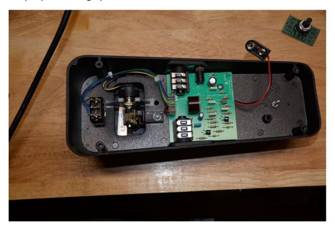
The stock circuit board assembly was removed leaving the existing DPDT footswitch and the (like new) pot in place. The stock clutch was removed and replaced with a new 3/8" nylon pipe clamp. Yes. This is a HILLMAN item that is sold at LOWES (and other stores) for \$1.04 for a package of 10. It looks and works just like the original DUNLOP clutch!
