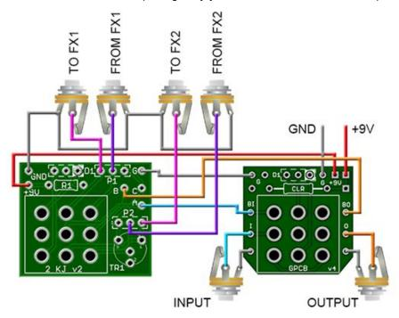
While the wiring for the signals must be followed, the power supply and ground wires can be routed in different ways e.g. the +9V wiring can be done as in the diagram or both wires can be run to the +9V supply (whichever is shorter), the ground wires for the jacks can be connected to either board or run directly from power supply ground, again, whichever is shorter.
