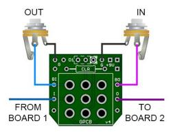
With this method any effects plugged into the effects loop are bypassed with a footswitch on your combo enclosure.
