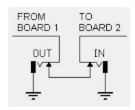
With nothing plugged into the jacks the signal passes from board 1 to board 2, when an effect is plugged into the jacks the signal passes through the effects.
