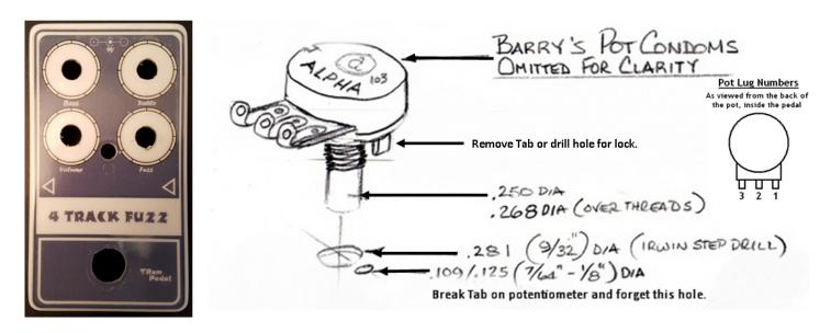
**Part 10: The Wiring.** Look at the pictures below. It is best to pre-wire your potentiometers and your foot switch. GuitarPCB also carries an excellent **3PDT Wiring Board** for a great price and keeps your wiring clean as well as allowing you to install either a Standard On/Off LED or one of their three different Bi-Color LEDs while keeping your power wiring and audio wiring separate.
