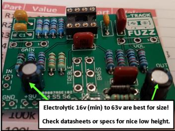
**Part 5:** I check over the entire board for good clean solder joints. If there are any questionable areas I can easily re-flow them now. Once satisfied with my work I can install the IC Chip into the socket. **The IC Chip also requires correct orientation.**
