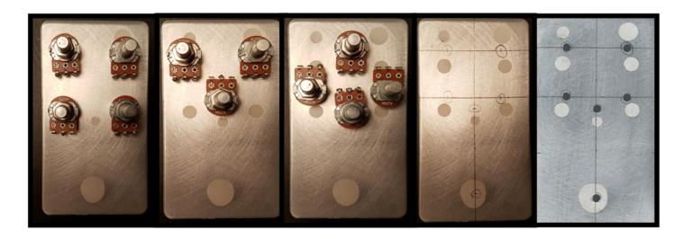
**Part 7: Laying out the design.** There are many ways to do things so you must decide what works best for you. In this case I placed the drilled enclosure in my scanner to import a picture into Illustrator or whatever program you like (GIMP is Free). I can begin to place knobs, LEDs, 3PDT switch, Input and Output Jacks as well as the power jack. This will give me a better idea about how I would like my pedal to look and make any changes "virtually" that may be needed.
