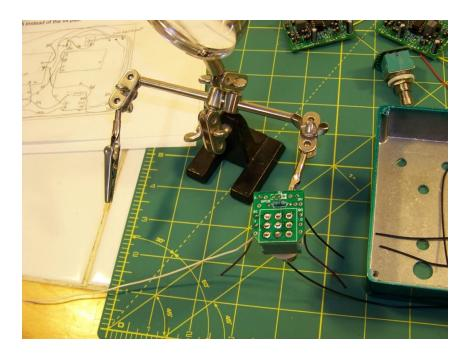
It's good to have several colors of wire to work with. It helps if you use a color for a certain purpose. If you can just look at a color and know what it does it helps tremendously. For example I chose white for the bypass signal from input, through each <u>3PDT Wiring board</u> and to the output. Violet was used for the board ins and outs. As you apply heat to the wires while soldering you will notice that the insulation will melt back slightly. That is normal.
