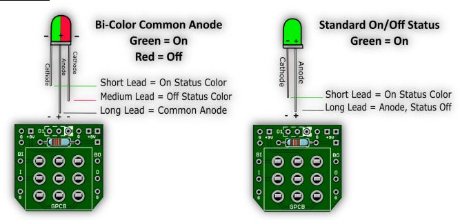
Note: If wiring the LED to our 3PDT board no need to connect S4, S5 & S6 or populate D1 or R5 (CLR) on the main board since you are wiring your LED directly to our board.
