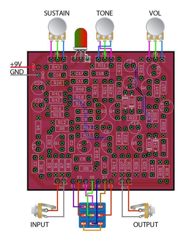
The standard circuit employs a buffer stage (Q1 stage) that is permanently connected even when the circuit is in bypass mode i.e. the circuit is not a true bypass system.
