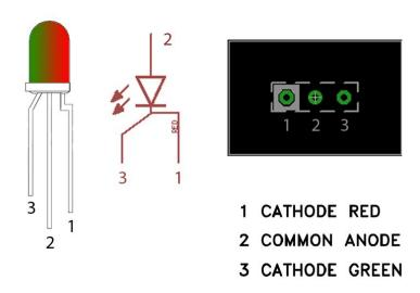
The diagram above shows the pin-out, schematic symbol and pad connection for a common anode LED. The pin-out for the bi-colour LED is as follows:
