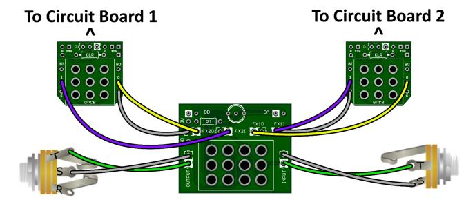
Using our 3PDT Wiring Boards in tandem with the Easy Order Switch makes it easy and neat to share power with other boards. No need for Star Grounding!!
