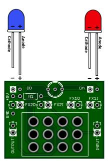
The bi-colored LED can be replaced with two standard LEDs as above Red is FX1 – FX2 and Blue is FX2 – FX1. Another alternative is to use just a single LED.
