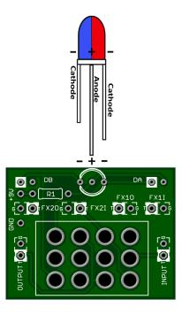
Using a Common Anode Bi-colored LED as shown above will result in the Red LED lighting when the effects order is FX1 – FX 2 and the Blue LED lighting when the effects order is FX2 – FX1.
