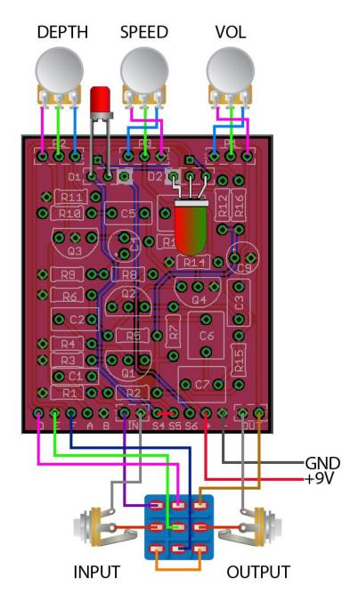
This method of wiring is for a circuit similar to version 2 of the EA Tremolo. It uses a standard LED for D1 and a bi-coloured LED for D2 for bypass switching status.
