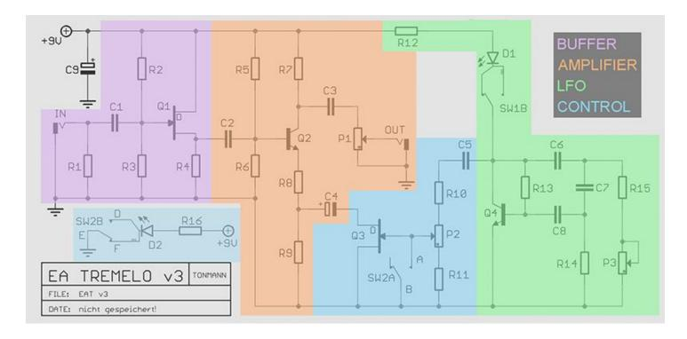
**Audio** - two stages, Q1 is a buffer stage which doesn't amplify the signal but "grabs" as much guitar signal as possible from the input and sends it to the second stage, Q2. The second stage amplifies the audio signal, the amount of audio signal gain for Q2 is controlled by the JFET, Q3.
