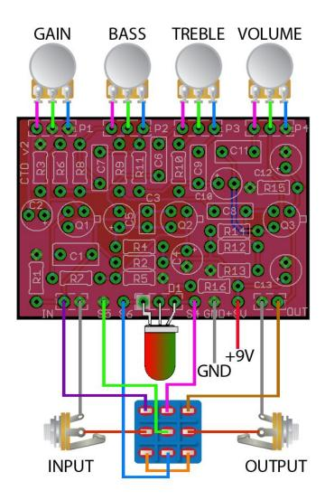
If you are using one of GuitarPCB's 3PDT Wiring Boards and choose to mount the LED to the wiring board instead, pads S4, S5, S6 and D1 would be ignored and R16 would not be installed.
