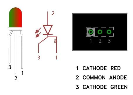
The diagram above shows the pin-out, schematic symbol and pad connection for a common anode LED.
