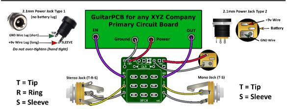
Multiple +9v and Ground Pads are convenient hookup points for additional circuits within the same enclosure. This also allows for diverse wiring schemes to suit indiviual needs.
